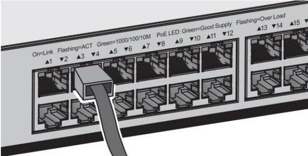
2. Configure the PC with an IP address 192.168.1.xxx. Please note that 192.168.1.200 is in use by the switch.
