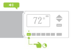
On the Wired Thermostat, press and hold the set button until the Wired Thermostat double beeps.
