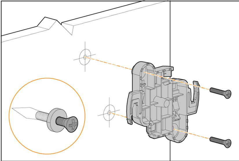
5. Align the access point with the mount bracket, placing the access point so that its mounting tabs are at an angle of approximately 30 degrees to the mount bracket.
