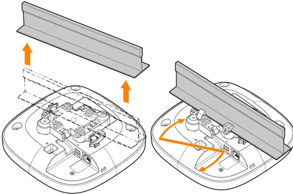
**Figure 5** *Installing Access Point to 9/16" Ceiling Rail*
